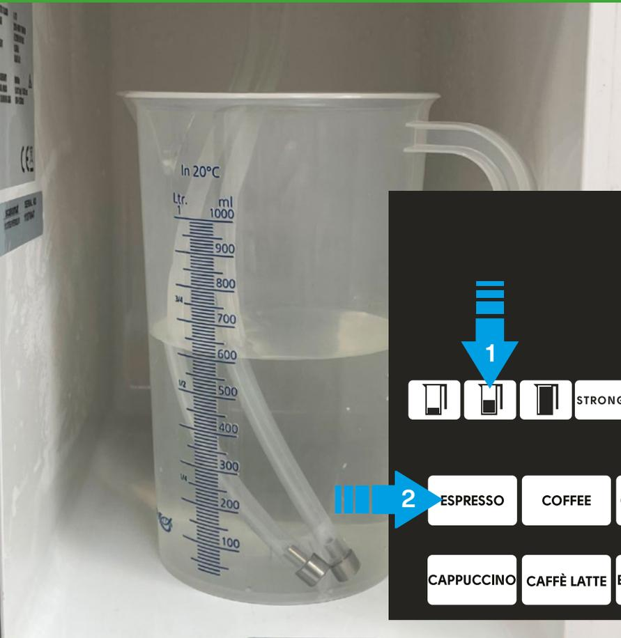
*On TopBrewer Compact push exactly the same buttons though the texts are different.*
